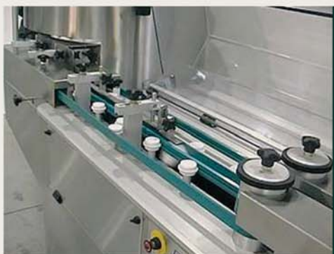
▲ Reinforced belts accurately control the movement and flow of bottles through the unscrambler.
